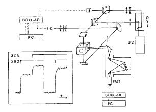
Fig. 2. Experimental diagram showing geometry used for smallsignal gain measurements and pump-dump experiments. Inset shows boxcar-averaged intensity levels obtained during gain measurement (see text for explanation).
