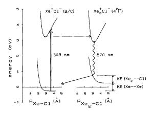
Fig. 1. Solid state energy level diagram showing states involved in four-level laser and disposal of kinetic energy after radiative dissociation (see text for details). Zero of energy is taken as the energy at infinite separation of the Cl atom from the xenon solid.
