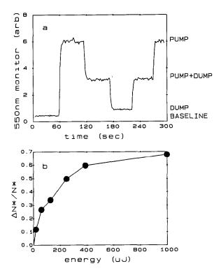
Fig. 4. Pump-dump signal levels from same sample as fig. 3. (a) Boxcar-averaged PMT signals with  $\lambda_{monitor} = 550 \text{ nm}$ ,  $\lambda_{pump} = 308 \text{ nm}$ ,  $\lambda_{dump} = 590$ , pump energy = 12 µJ and dump energy = 390 µJ. The dump only signal for 180 < t < 220 s does not return to baseline due to scattered 590 nm light reaching the PMT. (b) Fraction of excited state population that undergoes stimulated radiative dissociation versus dump laser energy.
