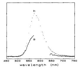
Fig. 3.  $Xe_2^+ Cl^-(4^2\Gamma)$  emission from a 1:1000 HCl: Xe solid at 12 K during 308 nm excitation observed with (a) and without (b) 590 nm dye laser dump beam. Monochromator slits were closed from 570 nm to 640 nm when using dump beam to avoid saturation of photomultiplier. Trace (a) is corrected for scattered 590 nm light and baseline.
