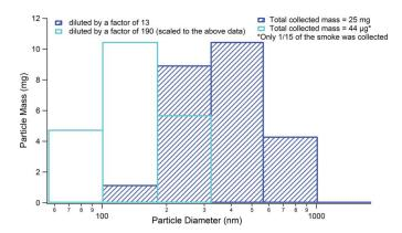
FIG. 7. Gravimetrically determined particle size distributions of e-cigarette-2 at two different dilutions: (1) dilution by 13, and (2) dilution by 190. The latter was close to the dilution used in the fast-flow tube experiments. The vertical axis corresponds to the data for the smoke diluted by a factor of 13; the data for the smoke diluted by a factor of 190 were scaled for the ease of comparison of the relative size distributions.
