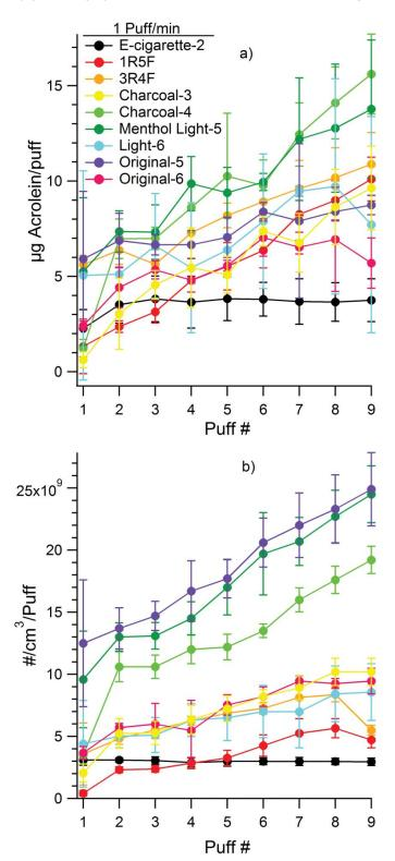
FIG. 4. Amount of acrolein (a) and particles (b) per puff for a puff frequency of 1 puff/min measured in fast-flow tube experiments.
