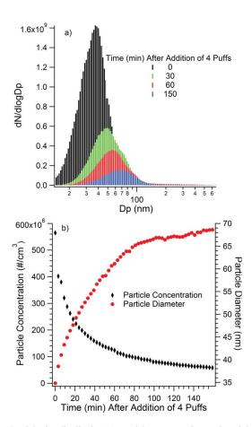
FIG. 3. Particle size distribution (a), particle concentration, and particle diameter (b), of e-cigarette-1 observed after injecting four successive puffs in a Teflon  $^{\text{TM}}$  chamber filled with zero air. The data were corrected for dilution to reflect the concentrations in the puff volume.
