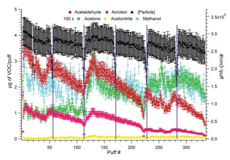
FIG. 8. VOC and particle content of e-cigarette-2 as a function of puff number during continuous use with a single cartridge (the battery was fully recharged at the beginning of vaping and at each interval (indicated by a line).
