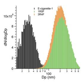
FIG. 2. Particle size distribution observed after injecting a single puff in a Teflon<sup>TM</sup> chamber filled with zero air. This data set was normalized to the total particle number concentrations data measured directly with the CPC and was then multiplied by the dilution factor.
