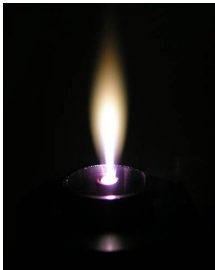
Figure 4.2. Argon MPT plasma with no nitrogen sheath flow. The candle shaped flame is caused by the flow of argon from the 1/4" tube. When a sheath flow is added, the plasma loses much of the tail flame and becomes thinner and more transparent.
