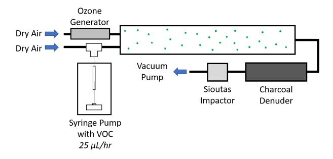
Figure 2.1. Diagram of the flow tube.
