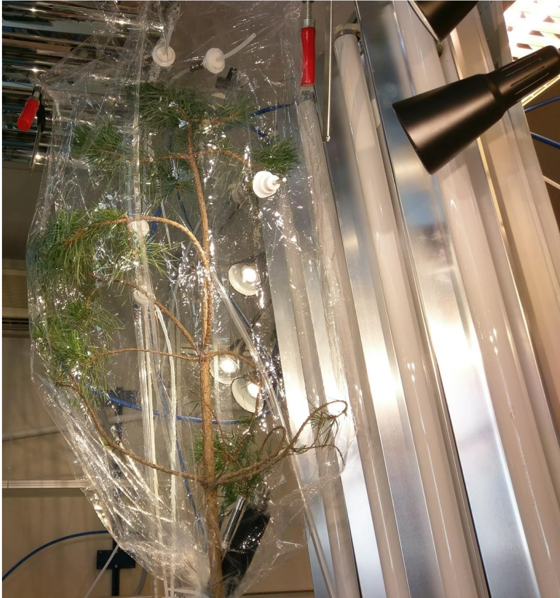
Figure 5.3. A photograph of the experimental setup wherein a tree sapling is placed inside the Teflon bag. The visible lights are turned on in this example.
