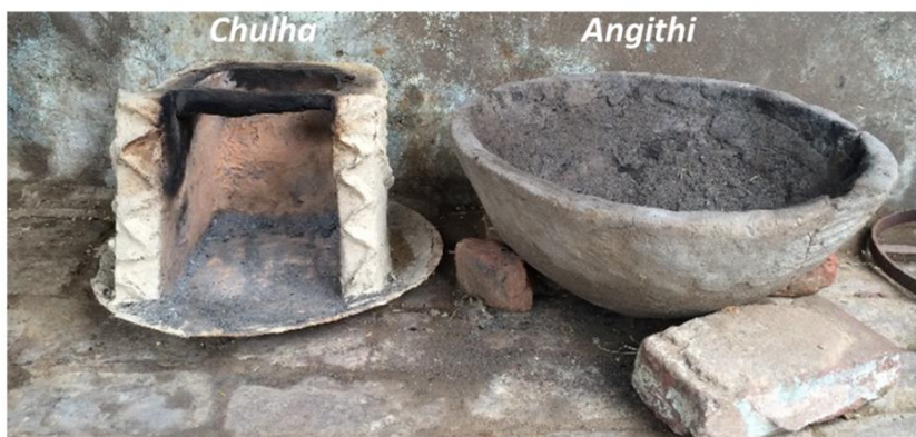
Figure 3.2: Stoves used in the study, the angithi and chulha , are pictured. Stove measurements and distances from the stoves to the inlet probes are found in the tables below.
