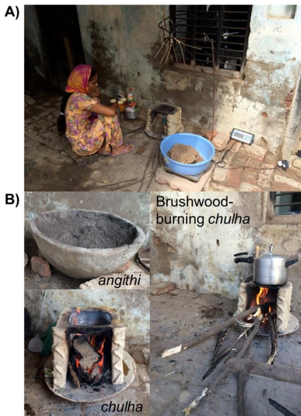
Figure 3.1: The field site and set-up for cooking events. A) The kitchen set-up at the field site. B) The stoves and fuels used in this study: angithi , dung-burning chulha , and brushwood-burning chulha .
